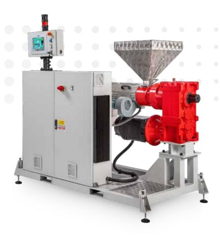
The RSZ series of extruders includes a range of machines with screw diameter from 45 to 90 mm and L/D 1:25 or L/D 1:30 depending on the kind of material.
