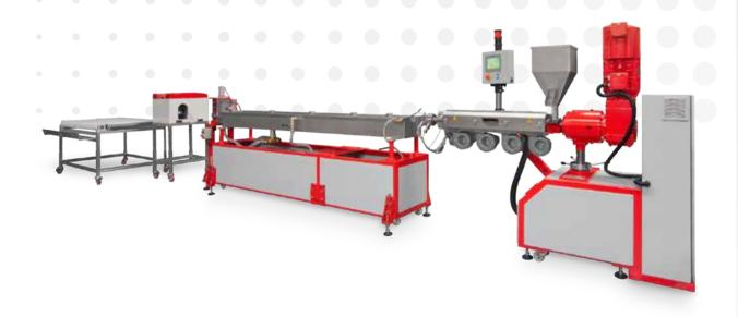
The attention paid to the definition of each of the individual components that make up the line, especially the profile of the plasticisation screws, temperature management, the identification of the cooling, pulling, cutting and collection system most recommended for a specific type of profile, has ensured that TeKnomast extrusion lines stand out for their reliability and performance.
