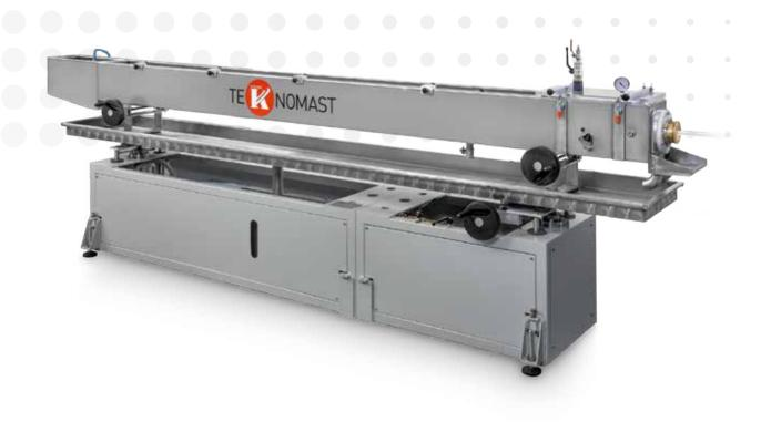
The tank type VRC, is indicated for the cooling and calibration of the HDPE, PP and rigid PVC pipes. All made by stainless steel, after the first vacuum zone, within which calibration occurs, is equipped by a tank where, in the first part the extruded product is cooled by immersion in water and, in the second, dried by a blast of air.
